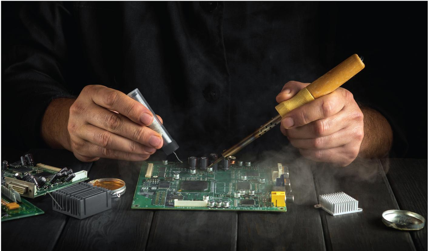
**Figure 8:** Besides automated soldering solutions, manual soldering is often necessary when a PCB component needs to be replaced.
