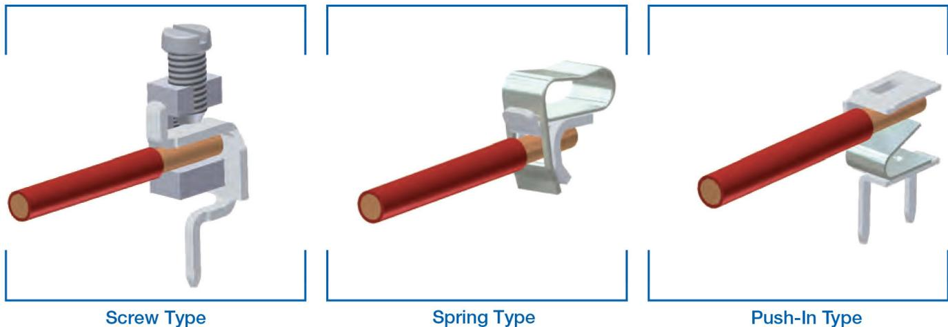
**Figure 2:** Illustrated are the three primary types of terminal block design.
