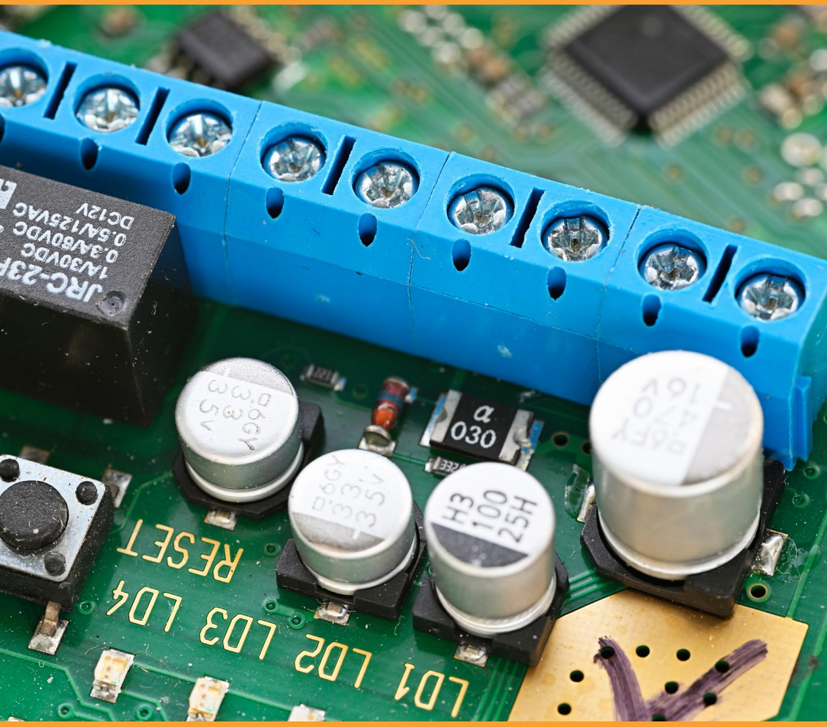
*Designing PCBs with terminal blocks requires an understanding of the types of terminal blocks available, the best way for them to be packaged for delivery, and how to solder them to reduce the potential for failure.*
